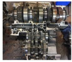
The rest of the motor still looked fantastic for the age and showed very little signs of wear. With the motor stripped the crank will be sent off to have new bearings and seals fitted. A job that could require up to a 50 tonne press to get the plates separated The crank took17 tonne to remove the plates!
