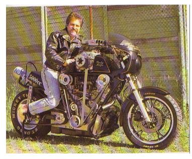
making the frame. He used a Holden gearbox and clutch, which the powerful engine destroys every couple of runs, and added a supercharger and nitrous oxide injector for good measure. The power the bike churns out is anybody's
